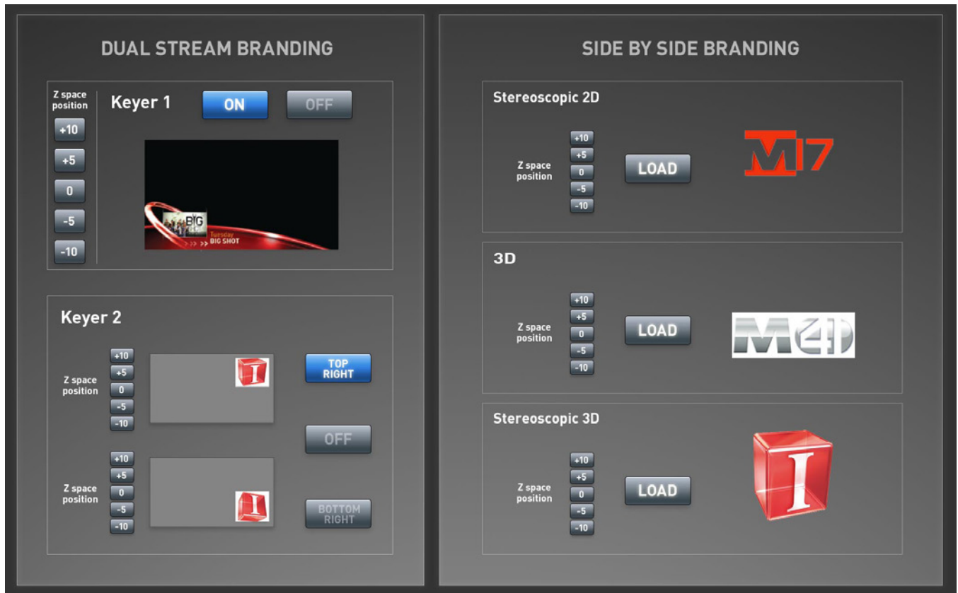
Picture 1. Stereoscopic 3D branding control panel with Z-axis-positioning control presets.
