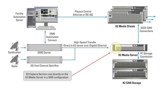
Figure 1 – Content is distributed over various networks into a catch server. Content is then directly transferred to the K2 system without transcoding resulting in 5-10 times faster than real-time transfers.
