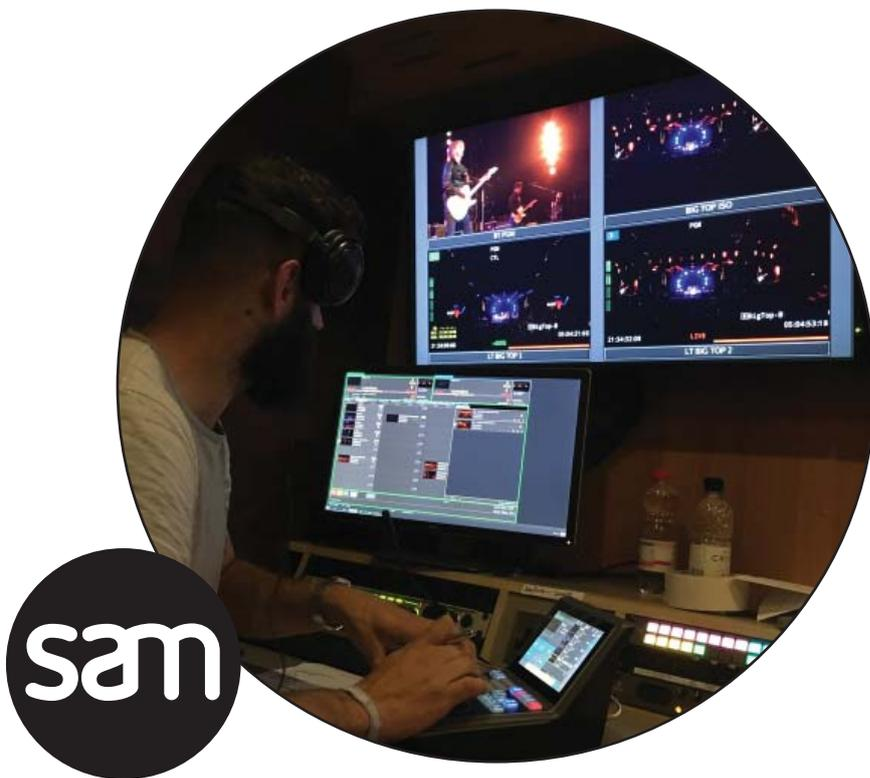
On the audio side, both a 5.1 mix and a downmix (LoRo) generated from each stage were sent to OB2's Calrec Apollo mixer for QC and routing. MADI from the Calrec, alongside the audio track from the music stages, was fed into a SAM Sirius 840 router. Embedding output cards were then used to record the eight tracks of audio in the first quadrant of the UHD Quad signal (i.e., 5.1 plus downmix). Greig explains that "having one frame from the downmix made things easier."
