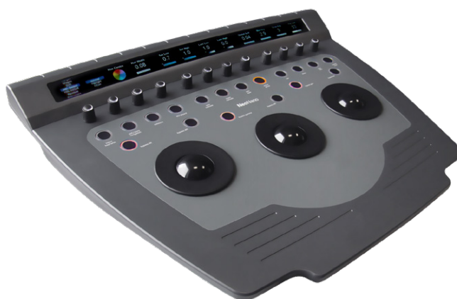
The Neo Nano Panel – Smaller footprint with 12 full-color OLED displays, and the same electroluminescent buttons, Neo Nano offers identical core primary and secondary grading options, user-definable presets and interactive visual feedback to the full-sized Neo Panel in a much more compact size.
