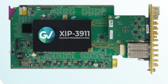
Densité 3+ XIP-3901-DC is an application that provide a dual-channel 12G/quad link 3G/3G/HD downconverter, which is designed to synchronize, downconvert and process 4K UHD 2160p and 1080p for both 1080p and HD broadcast production. The XIP-3901-DC application features broadcast-quality down-scalers, interlacers and color space conversions from ITU-R BT.2020 to ITU-R BT.709.
