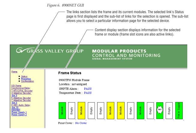
The 8900 modules can be addressed by clicking on a specific module icon in the frame status display or on a module name or slot number in the link list on the left.
