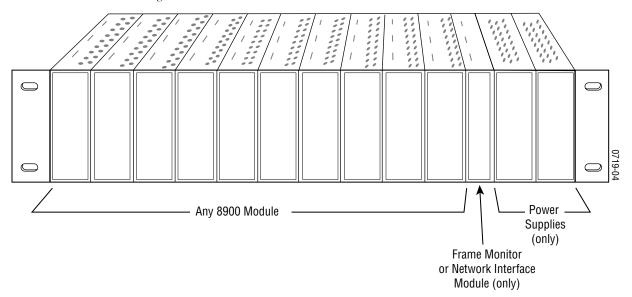
8900 modules are interchangeable within the module slots. There are 10 BNC connectors in each slot's I/O group. The functional assignment of each connector in a group is determined by the module that is placed in that slot. The maximum number of modules an 8900 frame can accept is ten. Figure 2 illustrates the rear connector plate for an 8900 Series frame.
