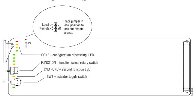
Figure 5. Module Configuration Switches and LEDs
