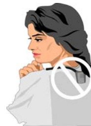
FIGURE 2.6 Sensor Blocked by Hair
