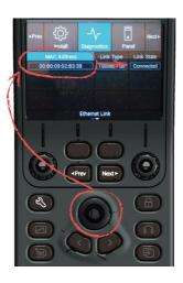
Push the central rotary to activate the selected setting. Turn the rotary to change its value and push again the confirm the new value.
