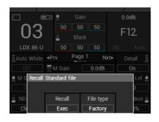
Use the right button below the display to select either Factory or Customer file to recall. Push the left button below the display to actually execute a Recall. Push the **Recall Standard** button again to cancel and close the popup window.
