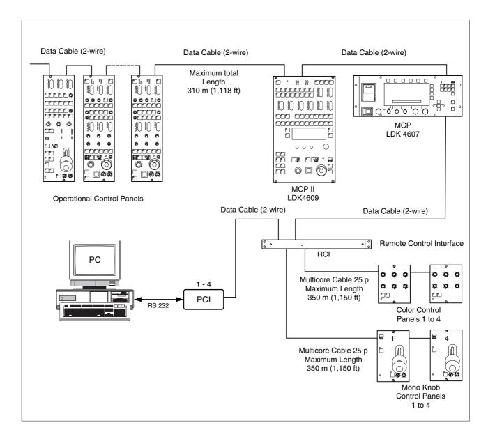
This configuration is the multiple camera Triax mode. The camera is connected to a CPU as in the single camera Triax mode. The data bus is looped-through from CPU to CPU's, Base Stations, OCP's and MCP. The OCP's (Operational Control Panels) are used to control the cameras and a MCP (master Control Panel) can also be connected to extend the control facilities.
