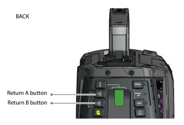
Return A and B buttons can be assigned to one of the three available External video channels or the teleprompter channel in the camera menu. Press and hold to view the assigned video channel in the viewfinder.
