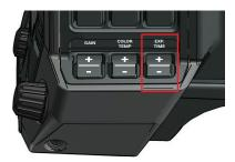
The exposure time switch gives a choice of exposure time settings. If an exposure time other than nominal is selected, the non-standard indicator in the (ocular) viewfinder lights.
