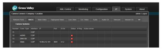
The **Conn.Type** column indicates the settings done in the camera(XCU). The interface that is using NMOS can be selected as well; it is either C2IP or Media. IP Address, Port Number, Version and Status are visible when a connection is made with the NMOS server.
