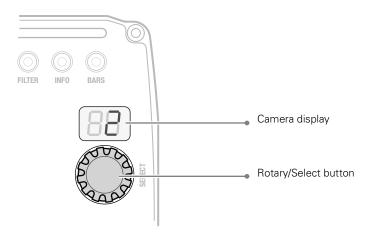
Press and hold the rotary/select button for a few seconds until the camera display starts flashing. Turn the rotary/select button to select the camera number from 1 to 99. Press the rotary/select button again to confirm the new settings.
