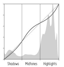
**OCP** Press the GAMMA button, the NEXT button, the NEXT button again and switch on CONTRAST. Select SHADOWS, MIDTONES or HIGHLIGHTS to adjust the luminance level for each range between 0 and 99.
