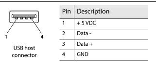
USB type A connector (host) compatible with USB 2.0 standard
