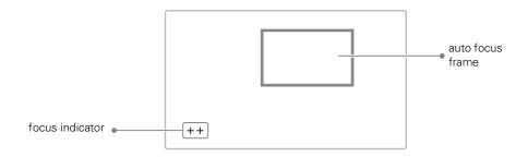
An indicator in the bottom left corner of the viewing output shows the current focus information:
