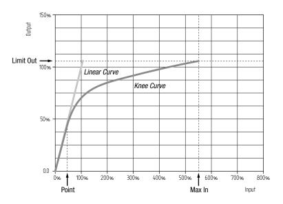
Knee can be set up as an automatic or variable function. It can also be switched off, which is the default setting.
