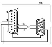
Auxiliary RS-422 (D-sub 15-pin (D-sub 9-pin female female connector) connector)
