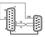
Auxiliary (D-sub 15-pin female connector)
