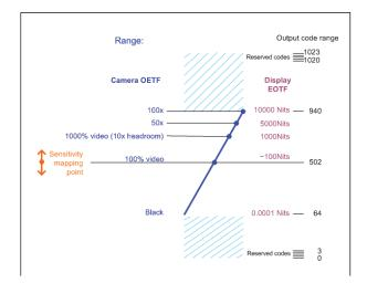
The camera's sensitivity can be mapped to either the SMPTE 2084/PQ or the HLG curve. The Sensitivity Mapping point can vary between 50% to 500%.
