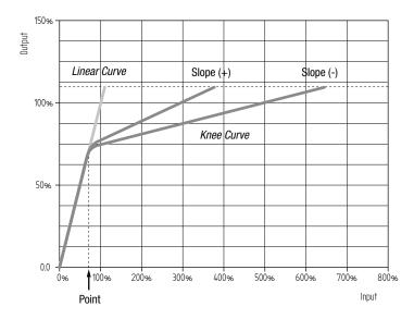
Knee can be set up as an automatic or variable function. It can also be switched off, which is the default setting.
