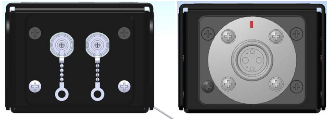
Fig. 3-5: SHED-C fiber-run side - ST connectors
