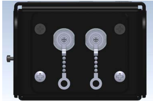
Fig. 3-3: Shed-BS fiber-run side - ST connectors
