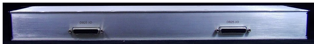
The rear panel has a DB25 connector for each input.
