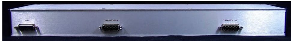
Fig. 2-7: Data-GPI panel - rear.JPG
