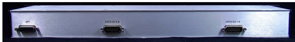
Fig. 2-9: Data-GPI panel - rear.JPG
