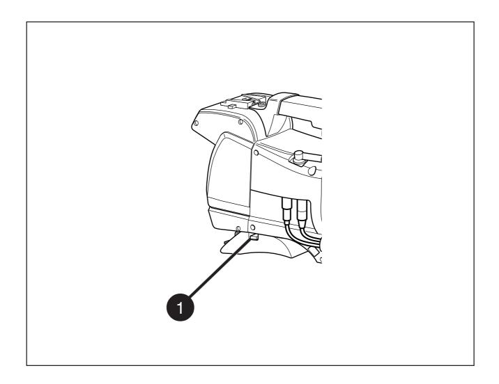
To change the position of the shoulder pad press and hold lever (1). The shoulder pad can now be moved backwards and forwards along the axis of the camera. Adjust the shoulder pad when all units have been mounted so that the best balanced position can be obtained.
