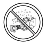
Avoid very damp places. If the environment is wet or damp a rain cover must be used to protect the unit.
