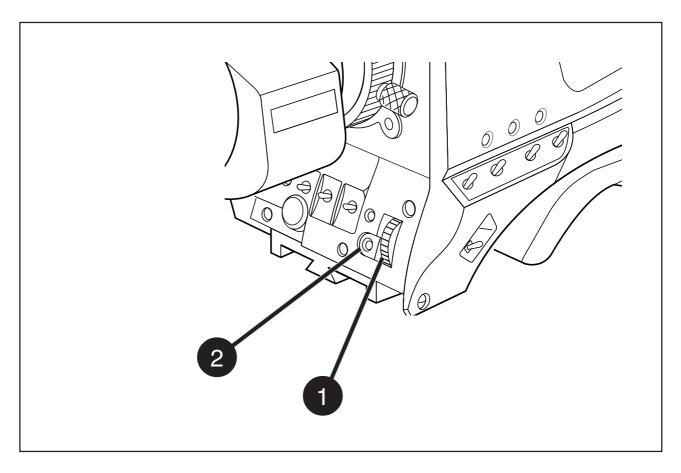
The system menus are displayed in the viewfinder. There are two controls at the front of the camera that allow you to navigate through these menus. The functions handled by the system menus are divided into eight different menus. Each of these menus gives you access to a particular group of functions. More information on using the system menus is contained in Section 6.
