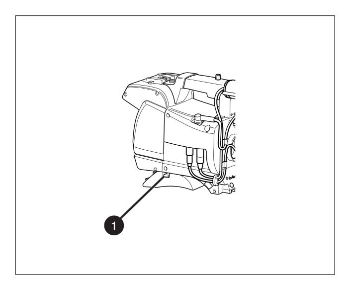
To change the position of the shoulder pad press and hold lever (1). The shoulder pad can now be moved backwards and forwards along the axis of the camera. Adjust the shoulder pad when all units have been mounted so that the best balanced position can be obtained.
