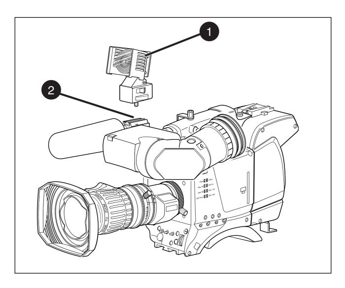
To mount a top light (1) onto the camera, proceed as follows:
