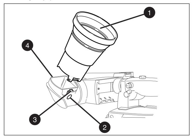
If you regularly use the viewfinder at a distance, for example, when you use the camera in the hand-held position, it is recommended that you fit the optionally available wide angle eyepiece (LDK 5390/00).
