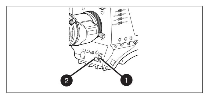
The system menus are displayed in the viewfinder. There are two controls at the front of the camera that allow you to navigate through these menus. The functions handled by the system menus are divided into eight different menus. Each of these menus gives you access to a particular group of functions. More information on using the system menus is contained in Section 6.
