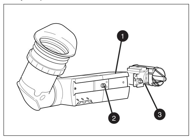
A left eye adapter is optionally available (LDK 5390/10) to allow the viewfinder to be used with the left eye.
