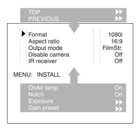
The Install menu above shows the items displayed when you first enter the menu and the other items that are available by scrolling up or down with the Rotary control.
