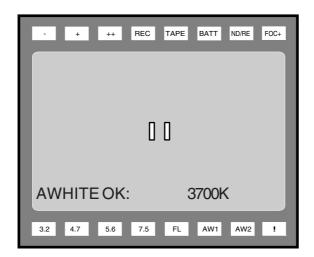
The measured colour temperature is now stored in the selected memory position and can be recalled as required.
