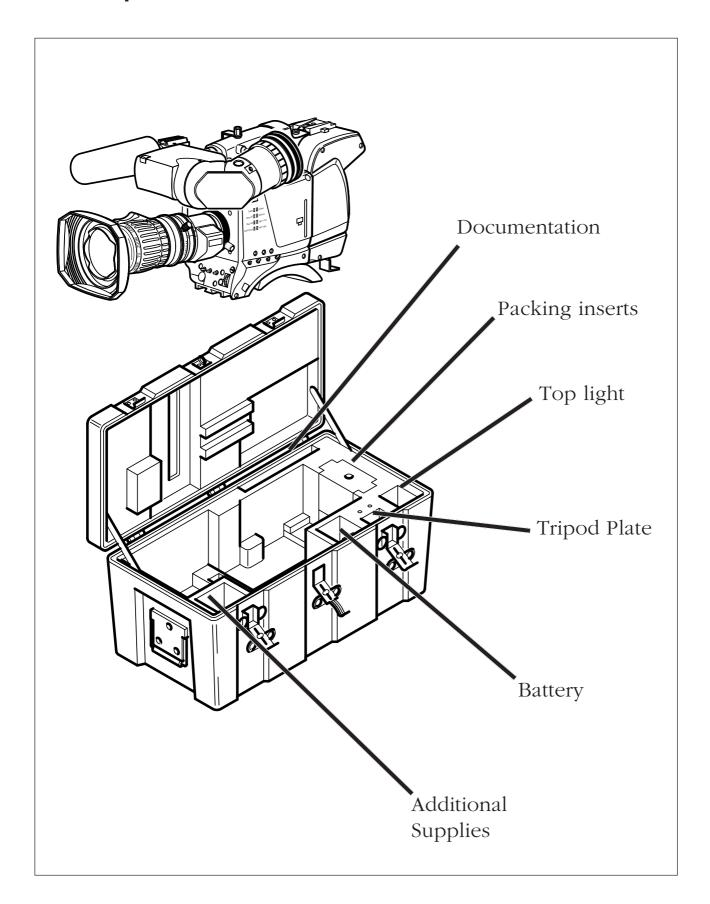
It is important to protect your camera against damage when transporting it. To do this, a transport case (LDK 5020/00) is optionally available for the camera, lens, viewfinder and some accessories.
