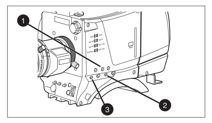
These buttons and switches only effect the monitoring signal and have no effect on the FilmStream output.
