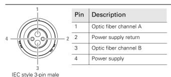
LEMO Hybrid Fiber connector compliant with SMPTE 304M.
