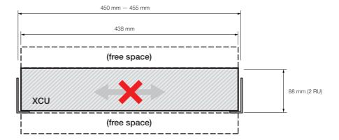
To prevent any vertical movement of the cradle during transport, lock up the cradle between other units and the vertical rail stands as indicated in the illustration below. Make sure there is enough support at the back of the unit, at a minimum distance of 400 mm from the rack front/
