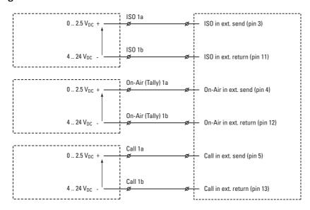
Apply a DC voltage to the inputs (respect polarity). If the voltage is low (0 to 2.5 V), the function is Active (or Inactive). If the voltage is high (4 to 24 V) the function is Inactive (or Active). The function state depends on the selection in the INSTALL > SIGNALLING INPUT menu:
