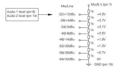
The actual audio level depends on the setting of the switches at the back panel of the camera adapter. When Mic is selected, the max. gain level is -64 dBu, while max. line level is -32 dBu.
