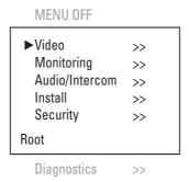
The main menu screen shows five items and the name of the menu (at the bottom). One or more item can be hidden but become visible when you scroll down. A cursor shows your position in the menu. Use the Up and Down buttons to move the cursor up and down.
