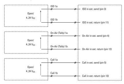
Leave the circuit open or apply a DC voltage to the inputs (respect polarity). If the circuit is open, the function is Active (or Inactive). If the voltage is high (4 to 24 V) the function is Inactive (or Active).
