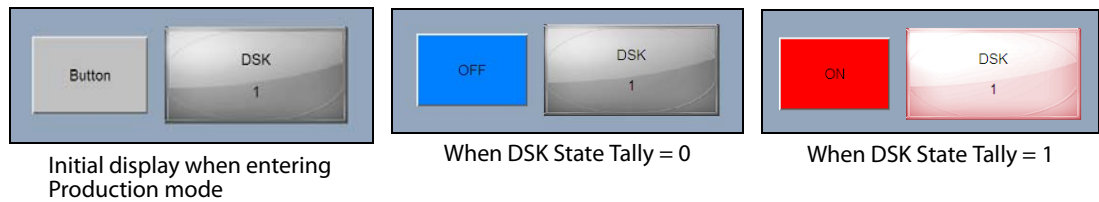
Fig. 5-2: The button's expected behavior in Production mode when a DSK State tally is received
