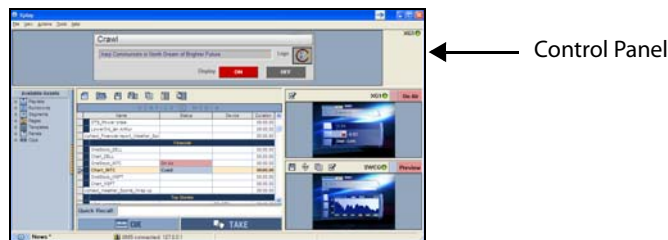
Fig. 4-8: Xplay can use a panel to playout and control graphics on an additional keyer layer
