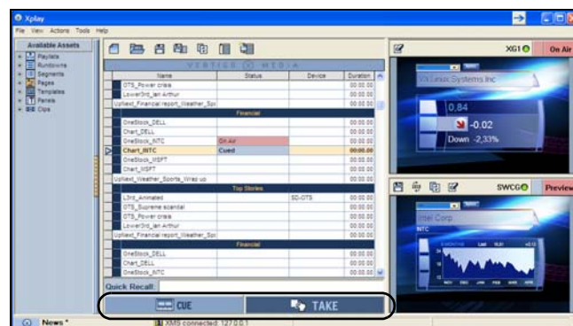
Fig. 4-3: Previewing cued playlist elements and then taking them to air on the playout device
