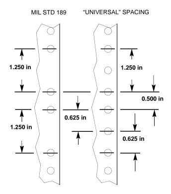
Front and rear rack rail mounting hardware is provided with the rack mount kit. Mount the rails using the enclosed hardware. Make sure the stationary sections are horizontally aligned and are level, as well as parallel to each other.
