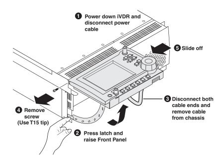
After the Front Panel is removed you can replace it with the Media Drive Door that is included with this kit.
