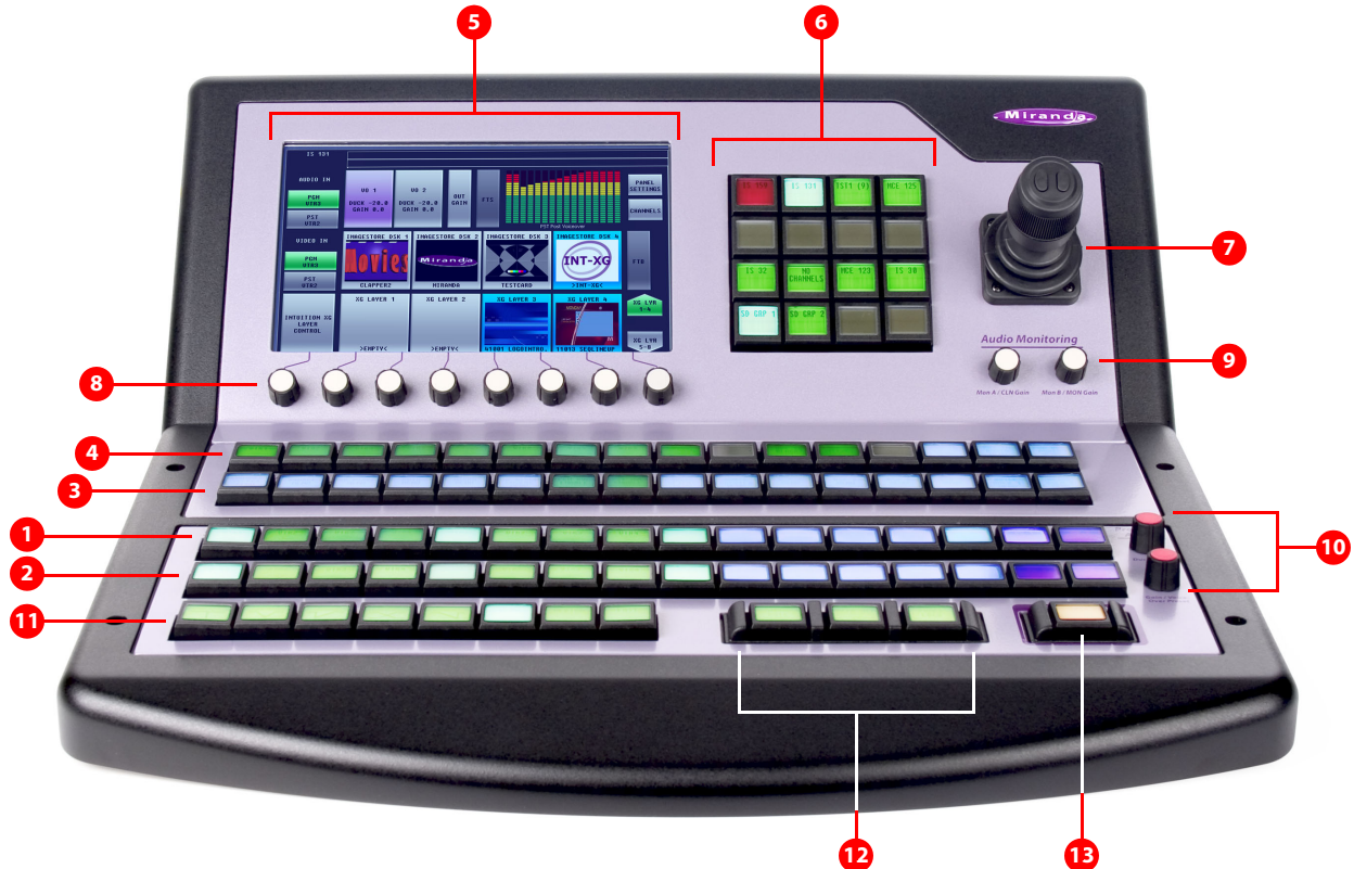
Figure 3-2. Sections of the iMC-Panel-200
