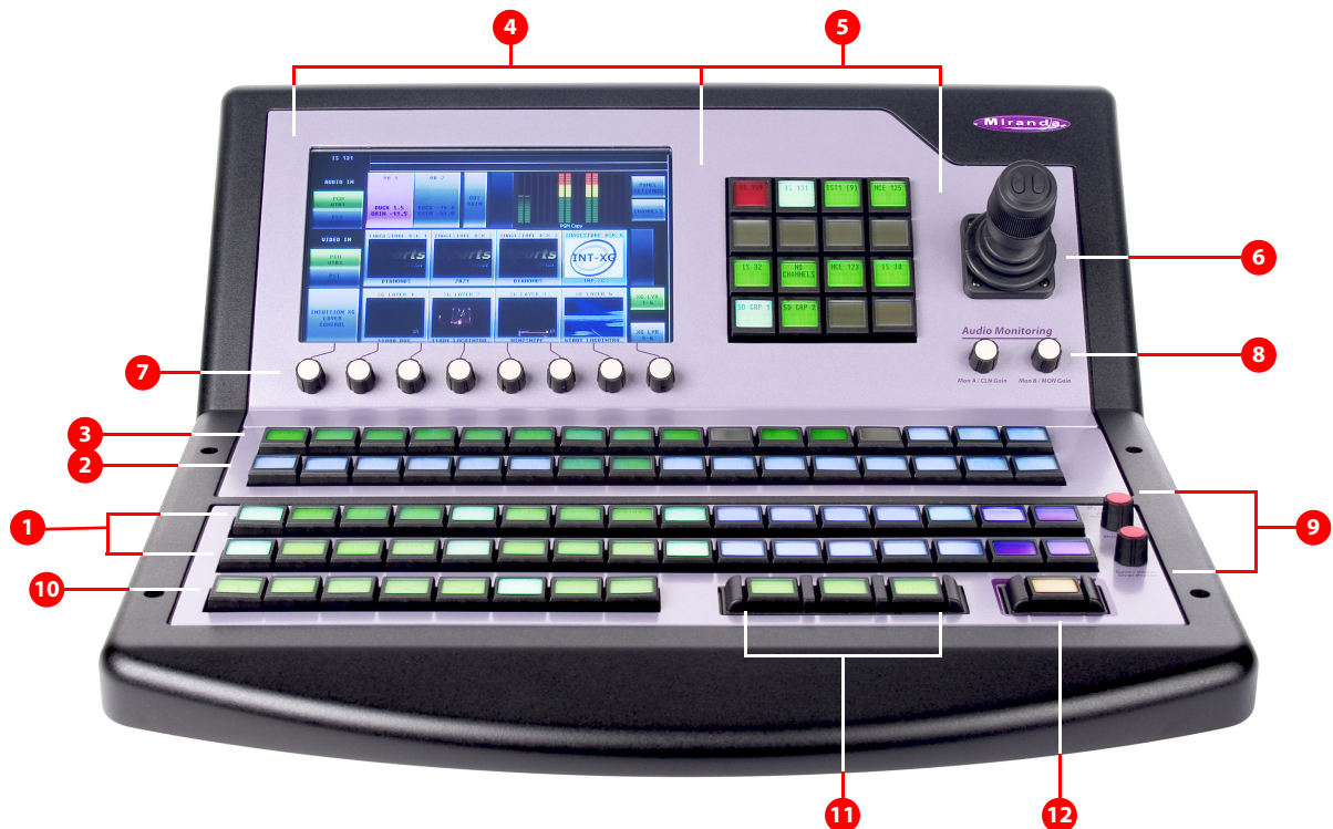
Figure 3-1. Sections of the iMC-Panel-200 (Shown Controlling an Imagestore 750)
