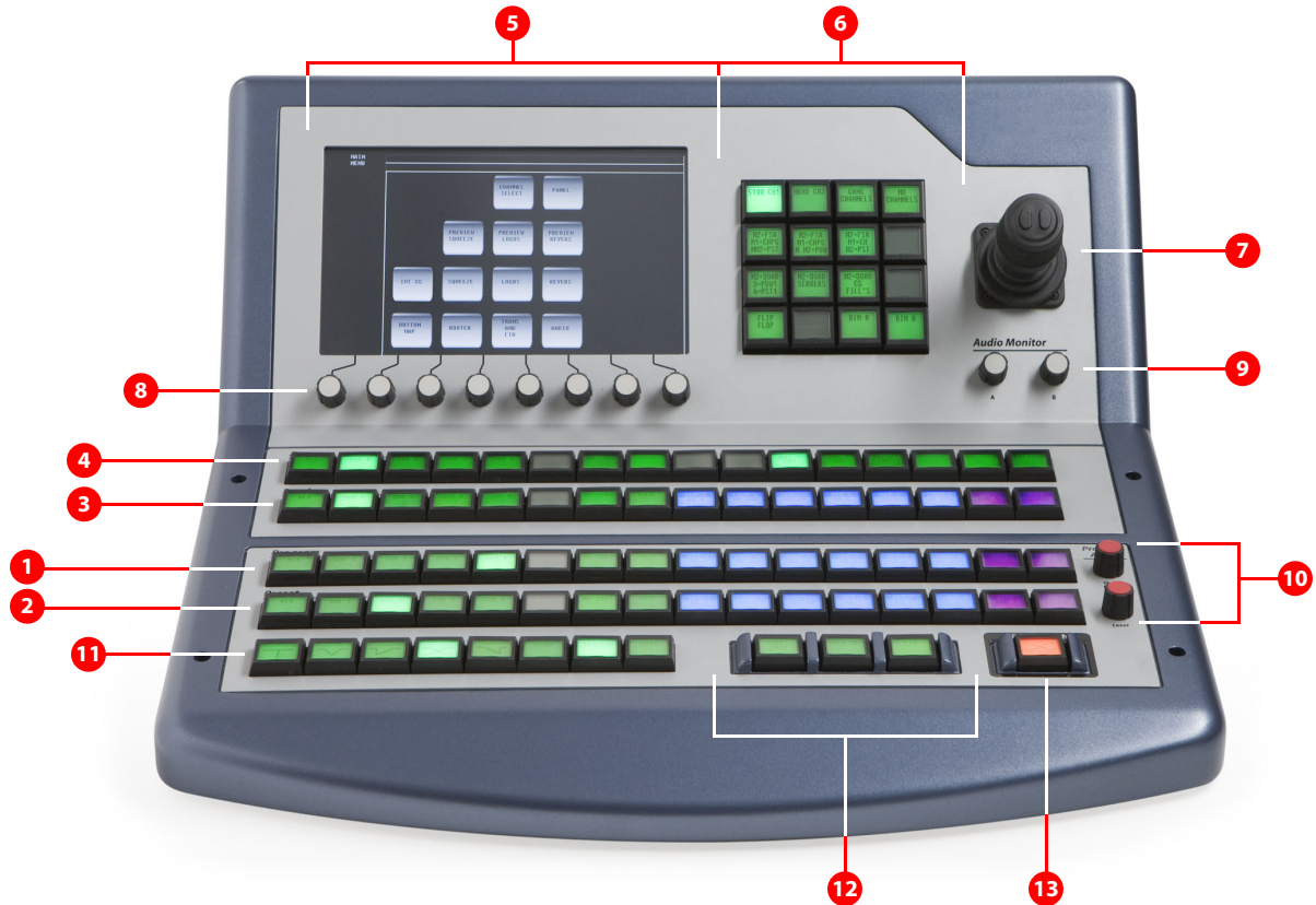
Figure 3-9. Sections of the CECP
