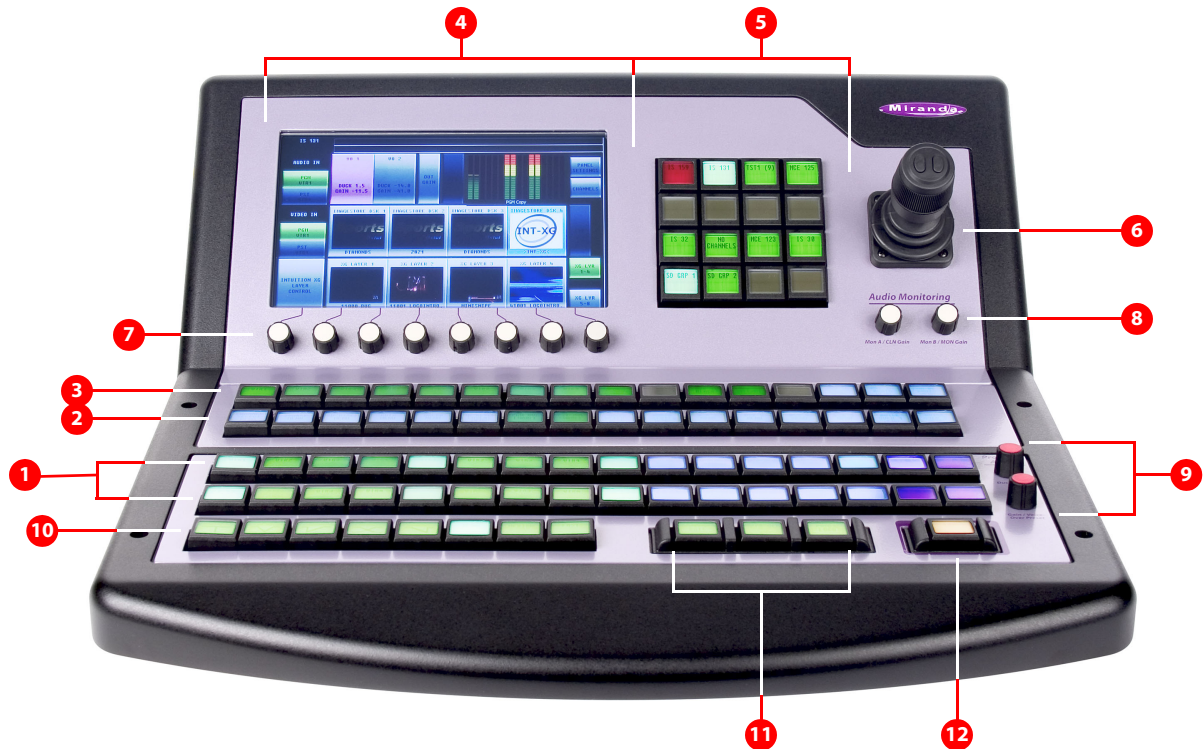
Fig. 3-1: Sections of the iMC-Panel-200 (Shown Controlling an Imagestore 750)
