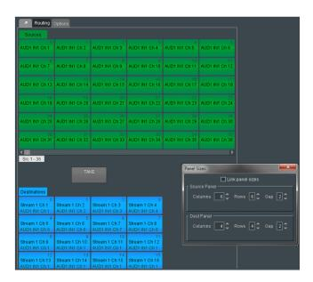
The GAP control adjusts the space between individual buttons:
