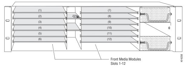
Figure 4. 2000T3 Frame, Front Slots
