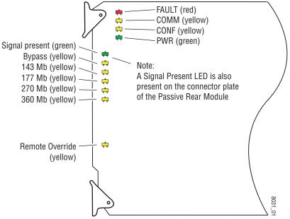
A red FAULT LED indicates an error situation and, when noted with the other indicator LEDs, can indicate a specific problem area. Table 1 describes signal output and LED indications for the various input/reference combinations and user settings.
