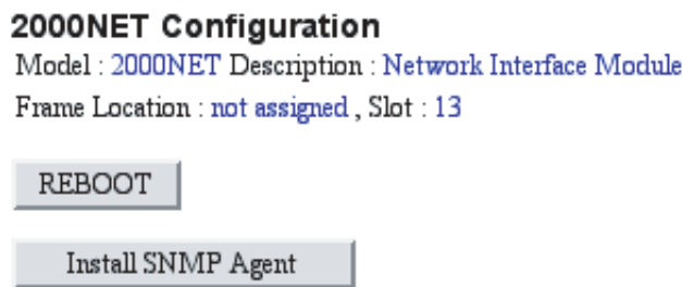
Figure 17. Configuring the 2000 Network Module for SNMP
