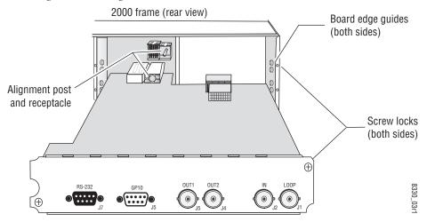
**5.** Locate the front slot 2, 4, 6, 8, 10, or 12 in the frame corresponding to the rear module circuit board. The 3 RU frame front view is illustrated in Figure 4 and the 1 RU frame is shown in Figure 5 on page 15.
