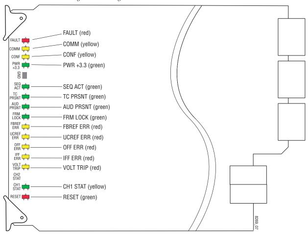
A red FAULT LED indicates an error situation and, when noted with the other indicator LEDs, can indicate a specific problem area. Table 4 describes signal output and LED indications for the various input combinations and user settings.
