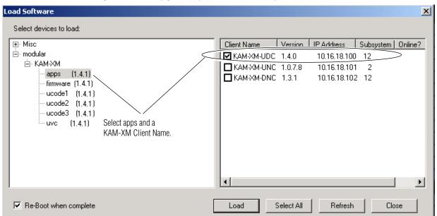
Figure 42. NetConfig Load Software Screen - First .fld Download
