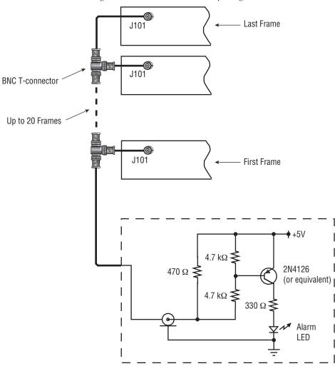
Figure 21. SMPTE Alarm Fault Reporting Connections
