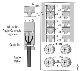
Figure 12. Audio Frame Rear Input and Output Connector Labeling
