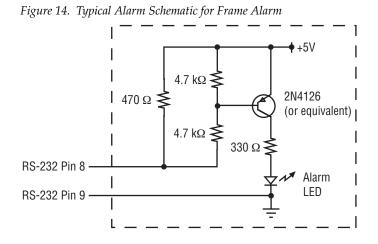
The impedance between the pins 8 and 9 of the RS-232 connector can be in one of two states:
