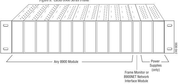
Figure 8. Gecko 8900 Series Frame
