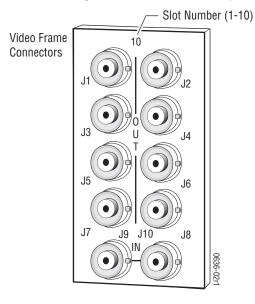
Figure 11. Video Frame Rear Input and Output Connector Labeling
