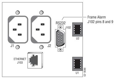
Figure 6. Power/Communication Connectors on 8900 Balanced Audio Frames
