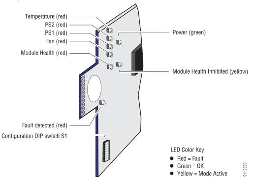
Figure 19. Frame Monitor Module Front View
