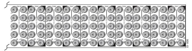
Figure 10 illustrates the 8900 Balanced Audio Frame three-terminal and BNC connectors on the rear backplane.
