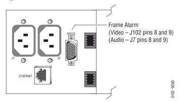
Figure 13. Frame Alarm Connector Location
