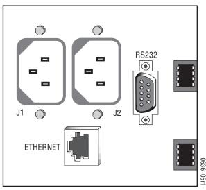
**Note** To maintain maximum redundant power, ensure that each power supply cord is plugged into a separate branch circuit.
