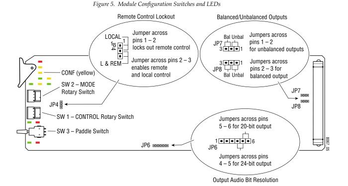
Table 6 gives the functions of each selection on the Control rotary switch (SW 1) and the action of the paddle switch (SW 3) in each function.
