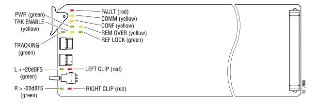
Figure 4. Operation Indicator LEDs
