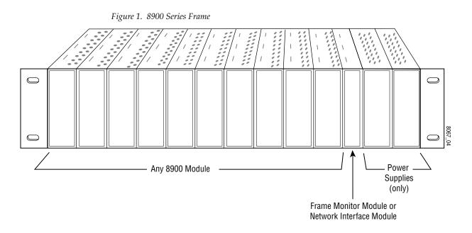
8900 modules are interchangeable within the module cells. There are 10 BNC connectors in each cell's I/O group. The functional assignment of each connector in a group is determined by the module that is placed in that cell. The maximum number of modules an 8900 frame can accept is ten. Figure 2 illustrates the rear connector plate for an 8900 Series frame.
