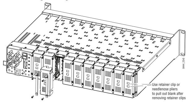
Figure 3. Installing Rear Module
