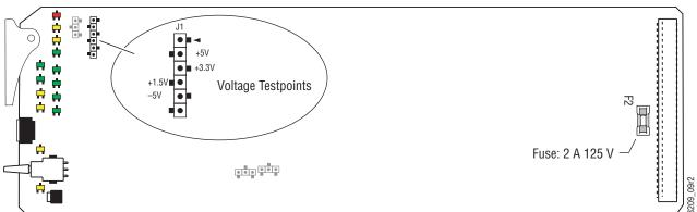
Figure 32. 8964ENC Fuse and Voltage Testpoint Locations
