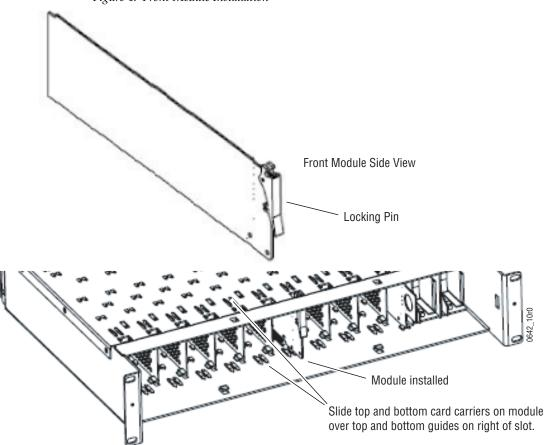
Figure 4. Front Module Installation
