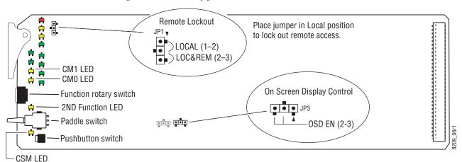
Figure 10. Module Configuration Switches and LEDs
