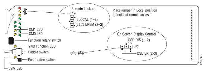
Figure 6. Module Configuration Switches and LEDs
