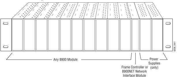
8900 module slots are interchangeable within the frame. There are 10 BNC connectors in each slot's I/O group. The functional assignment of each connector in a group is determined by the module that is placed in that slot. The maximum number of modules a Gecko 8900 frame can accept is ten. Figure 2 illustrates the rear connector plate for a Gecko 8900 frame.
