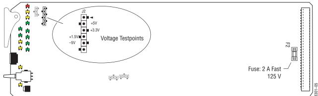
Figure 26. 8964FS Fuse and Voltage Testpoint Locations
