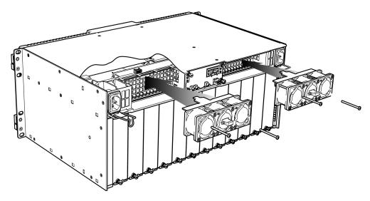
• Use the two screws that were retained when the old fan assembly was removed to secure the new fan assembly to the rear panel.
