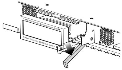
4 Pull gently on the display panel and slide the controller out of the frame.
