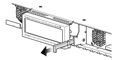
3 Push the lever firmly down to release the controller so that it can slide freely.
