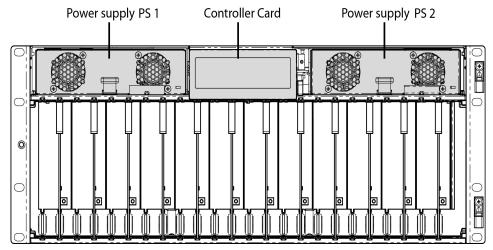
When the frame door is closed, the controller card touch screen is exposed through an opening in the top center of the door. All other front elements are concealed by the door.
