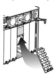
3 Slip the top of the 2RU rear panel into the slot on the bottom of the adapter, and secure the panel to the frame using the captive screw at the bottom of the panel.
