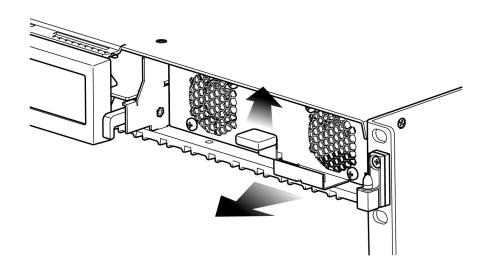
To install or change a power supply module:
