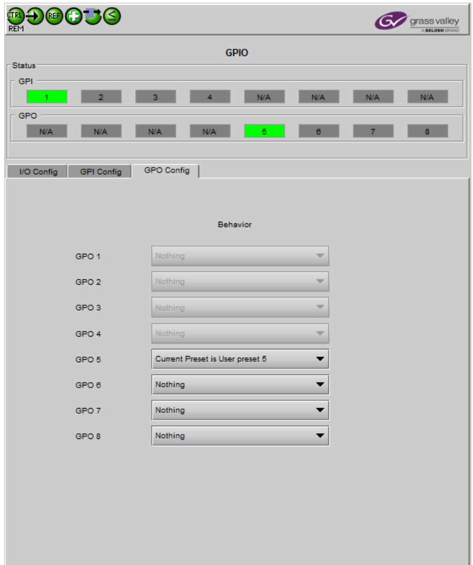
Figure 5-37 GPIO Panel - GPO Config tab
