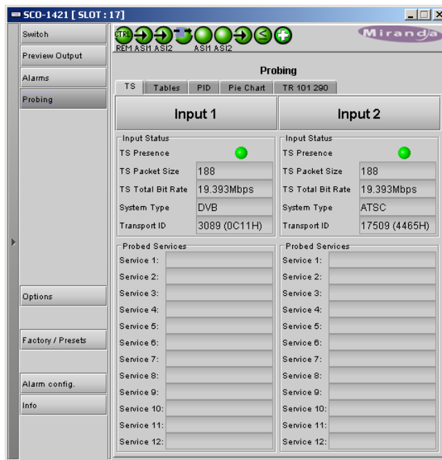
Figure 3.35 Probing – TS panel
