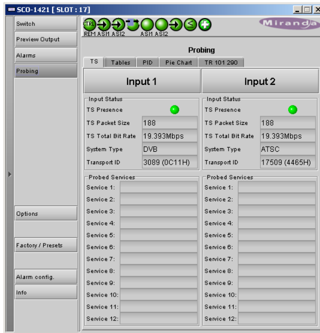
Figure 3.35 Probing – TS panel
