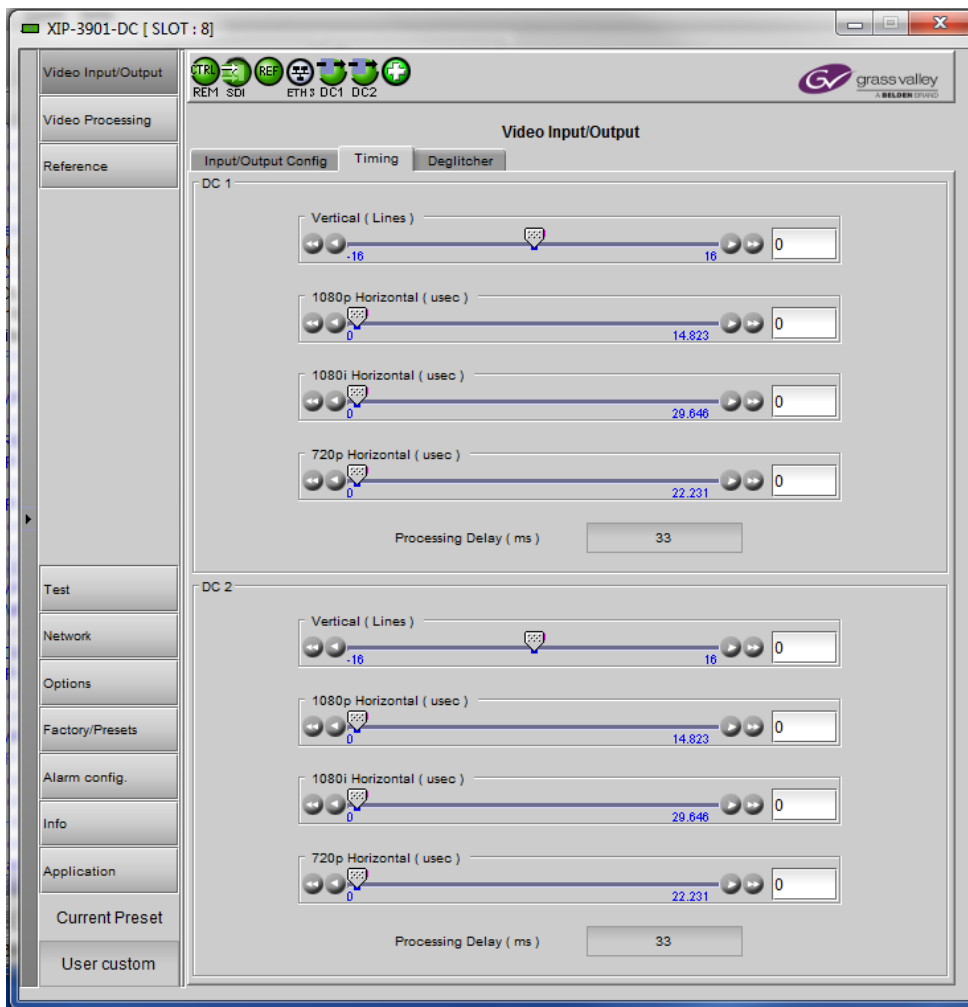
Figure 26 – Video I/O Timing
