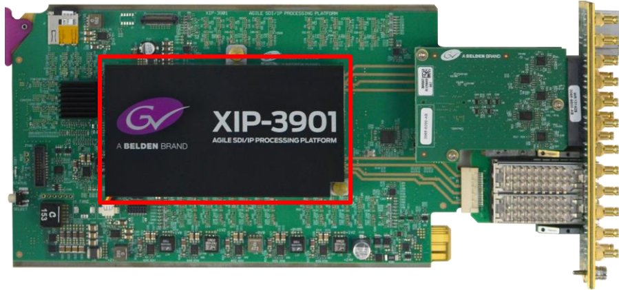
Figure 103 —Fan Assembly on the XIP-3901 Card
