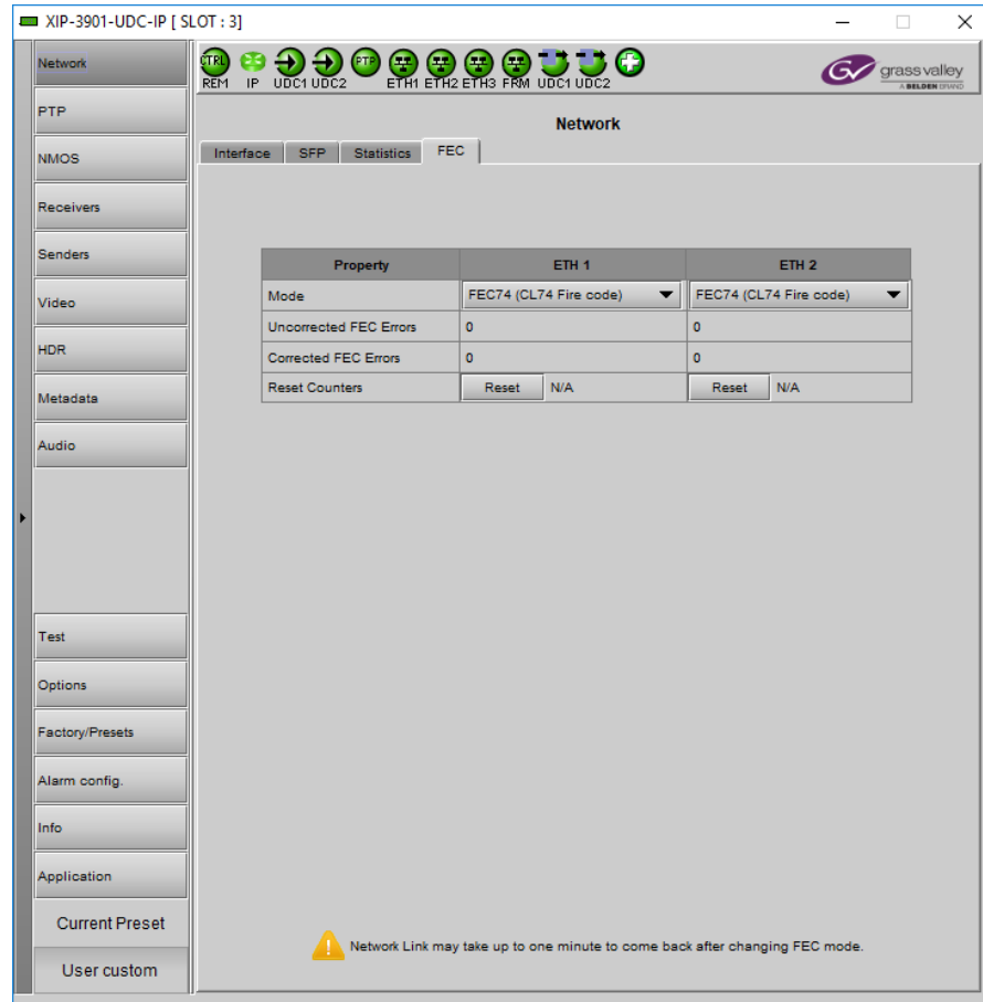
Figure 8-4: Network FEC Tab
