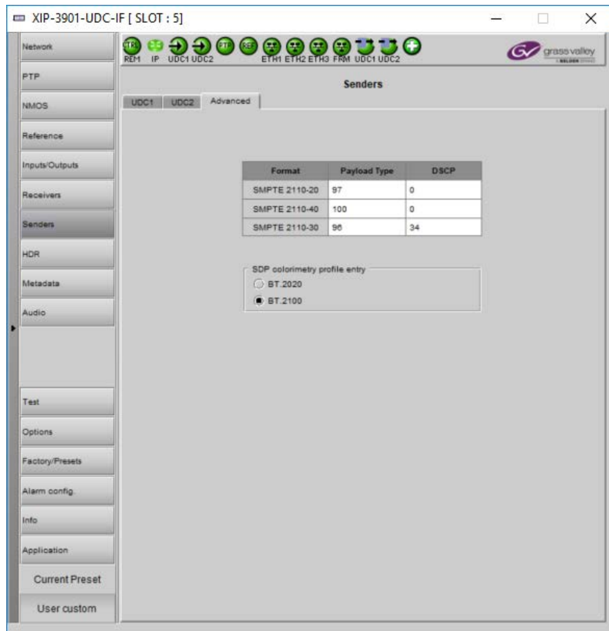
Figure 9-13: Senders Advanced Tab
