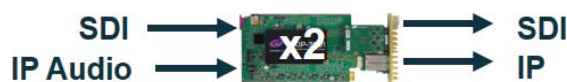
Figure 2-9: XIP-3901-UDC-IF Operating in SDI and IP Hybrid Mode with IP Audio Inputs
