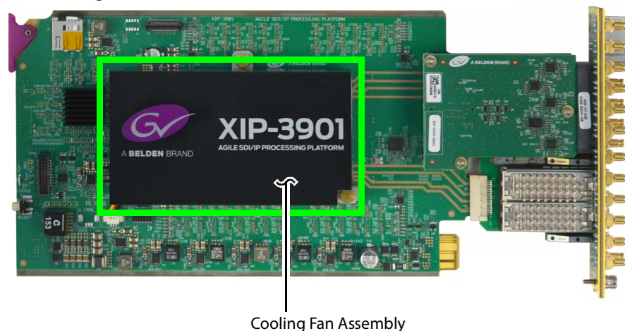
Fig. 14-1: Fan Assembly on the XIP-3901 Card
