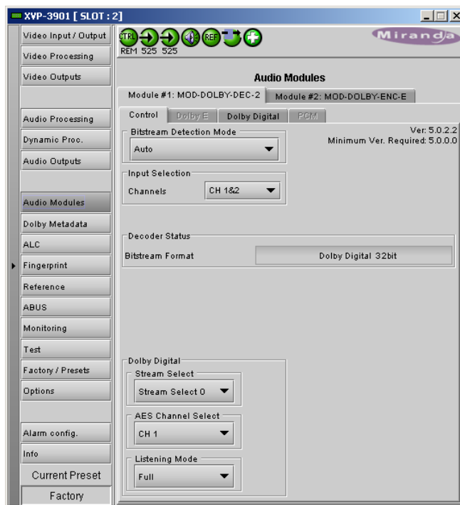
Figure 6.1 Audio Modules - Dolby Decoder - Control
