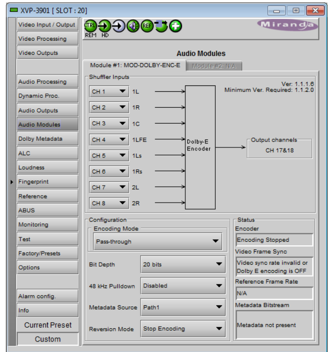
Figure 6.6 Audio Modules - Dolby E encoder
