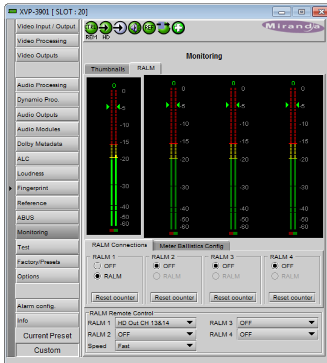
Figure 5.78 Monitoring - RALM tab
