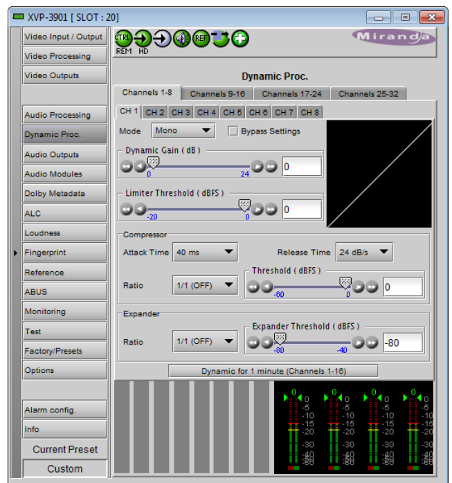
Figure 5.48 Dynamic Processing panel
