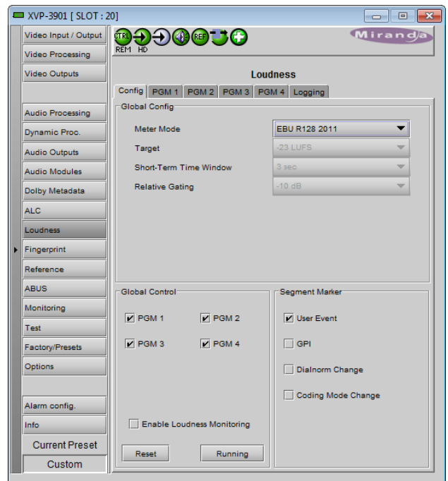
Figure 5.70 Loudness panel – Config tab
