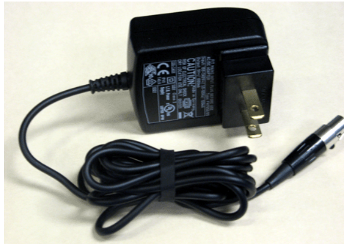
Figure 5. Standalone Power Supply-VMC-PS-D
