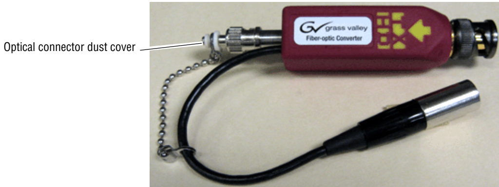
Figure 6. Video Media Converter (VMC) –Transmitter
