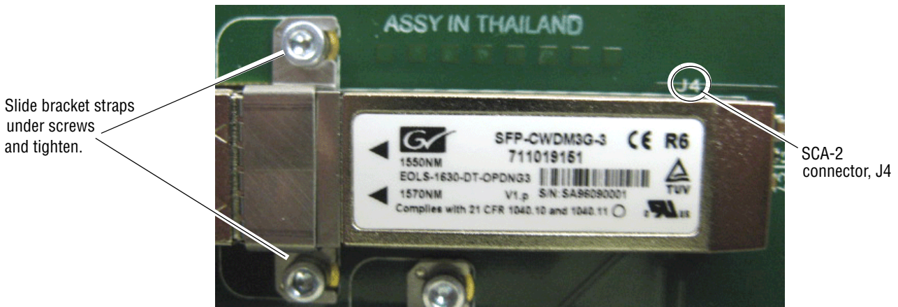
Figure 11. SFP Device Installation for Ch 3 and Ch 4
