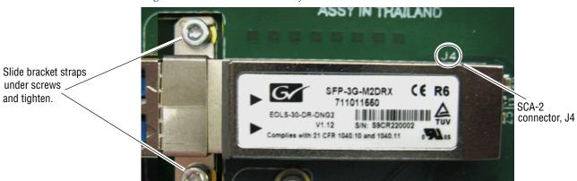
Figure 11. SFP Device Installation for Ch 3 and Ch 4
