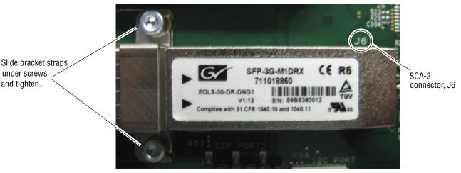
Figure 8. Installing F1 and F2 SFP Devices
