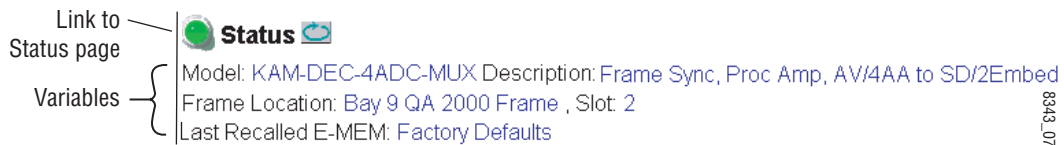
Figure 12. Typical Status/ID Header
