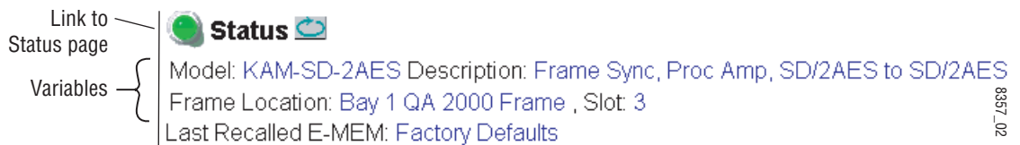
Figure 9. Typical Status/ID Header
