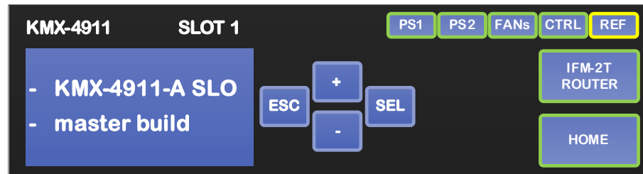
CPU-ETH3 local control panel
