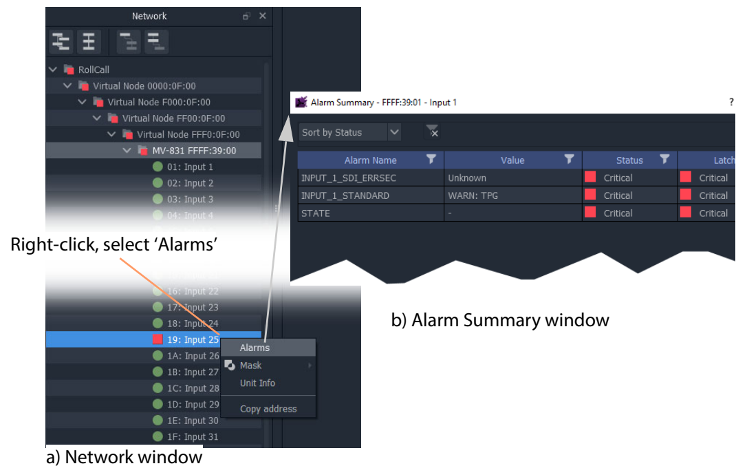
Fig. 7-29: Alarm Showing in: a) Network Window. b) Alarm Summary Window.
