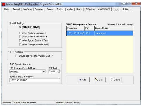
c With the ENDEC Manager Server added, select the **Enable SNMP** option and specify the IP Address in the **Operator Static IP Address** field.
