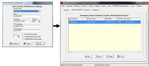
5 Click **OK** in the Encode/Decode Configuration dialog and the device is added.
