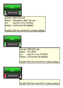
Regardless of the service's or channel's state, you can double-click the status button to display the **Service Provider Status** dialog, which provides even more details. Click the **Run Self Diagnostic** button to run and display a Diagnostic Report.
